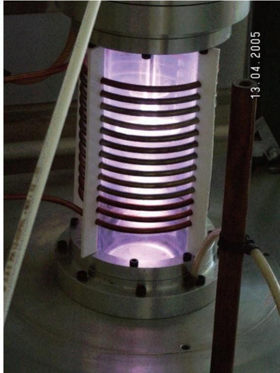
Figure 2: The discharge chamber of the 3l hydrogen plasma reactor
