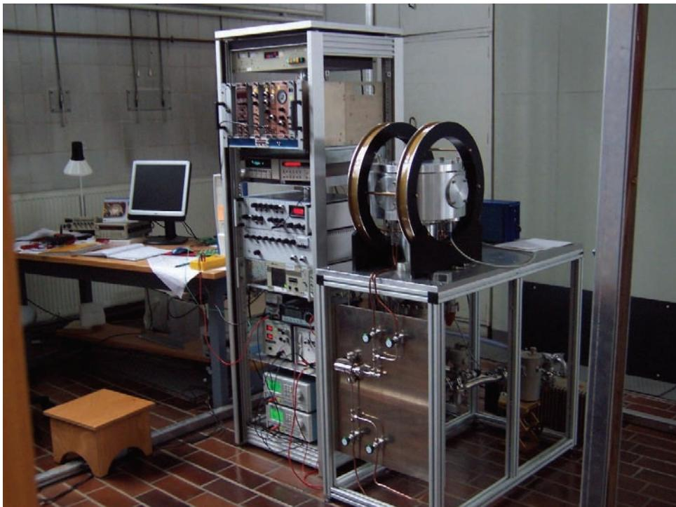
Figure 1: The vibrational spectrometer is housed in the vacuum chamber between Helmholtz coils that generate the homogeneous magnetic field needed for e-beam collimation and ion extraction.
